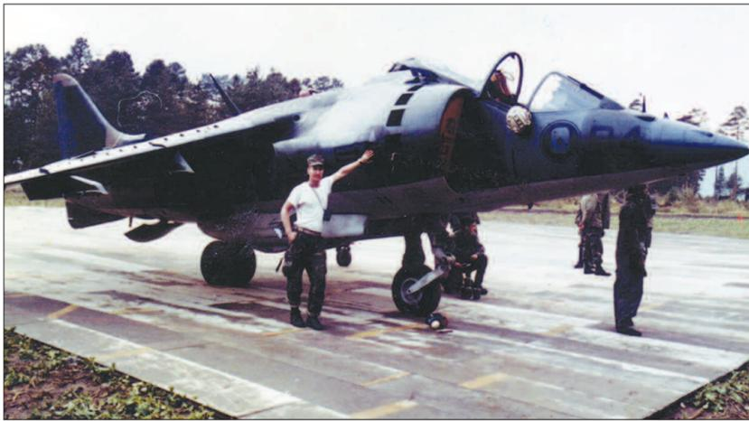
U.S. Marine Cpl. Mark Millican's squad of combat engineers built a portable landing pad for the Harrier "jump jet" during field operations in Norway in October 1980. Several Marine and Navy pilots died trying to learn to fly the aircraft, which lifts off vertically with two fore and two aft thrusters that rotate 90 degrees to the rear for forward flight.
